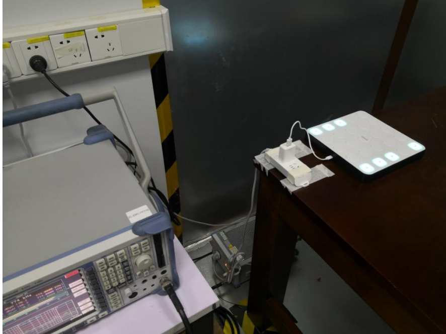
Conducted Emissions at AC Power Line (150kHz-30MHz)
