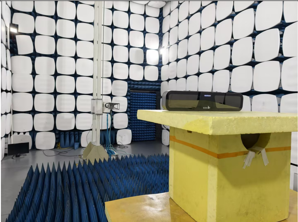
Radiated Spurious Emission, Above 1GHz
