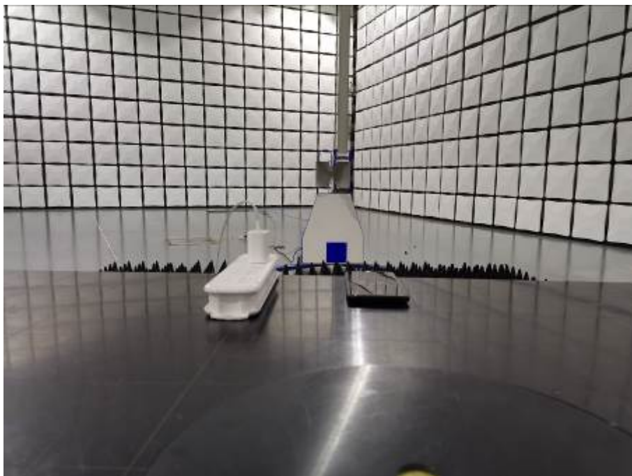
Radiated Emissions Test Setup (above1GHz)
