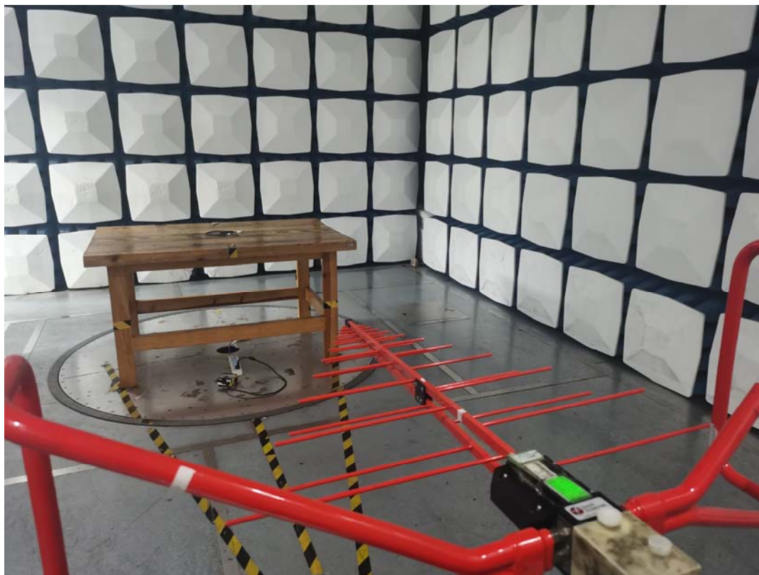
Radiated Emission Above 1GHz View
