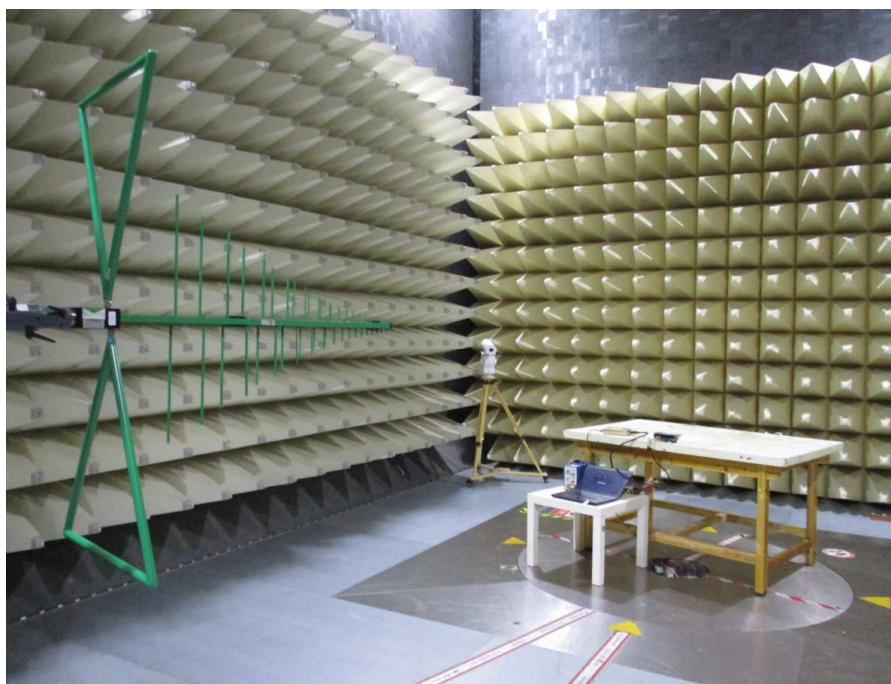
Photograph 1: Set-up for measurement of radiated emission
