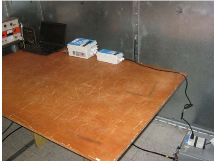
Figure 4. Conducted Emission from AC Line Test
