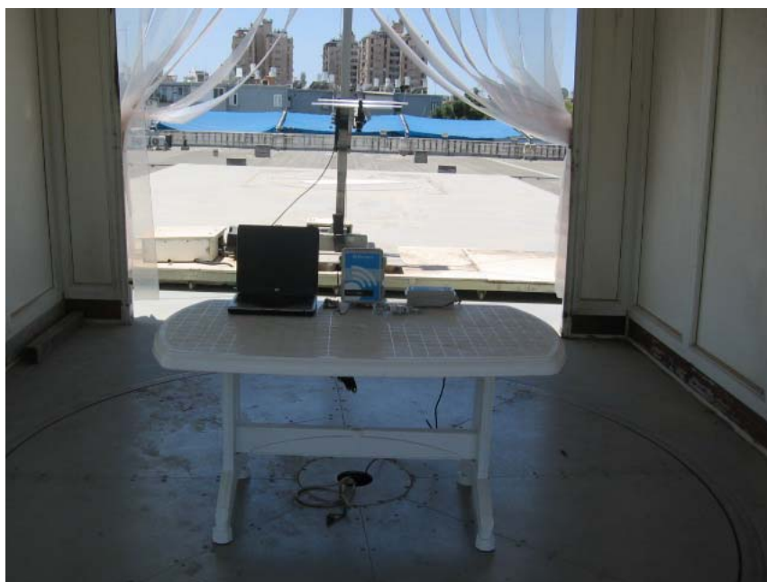
Figure 7. Radiated Emission Test, 200-1000MHz
