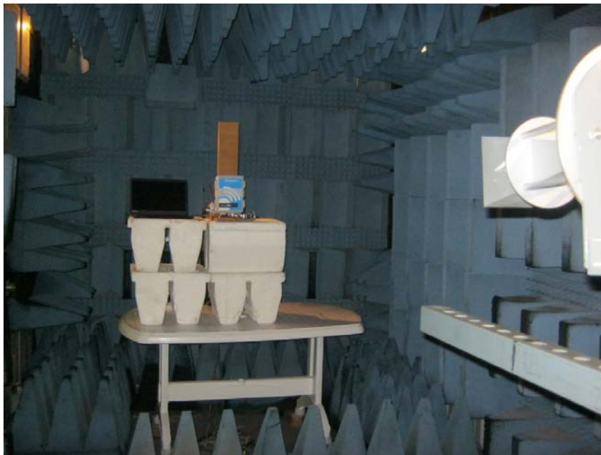
Figure 9. Radiated Emission Test, 18-26.5GHz
