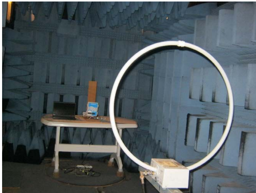
Figure 5. Radiated Emission Test, 0.009-30MHz
