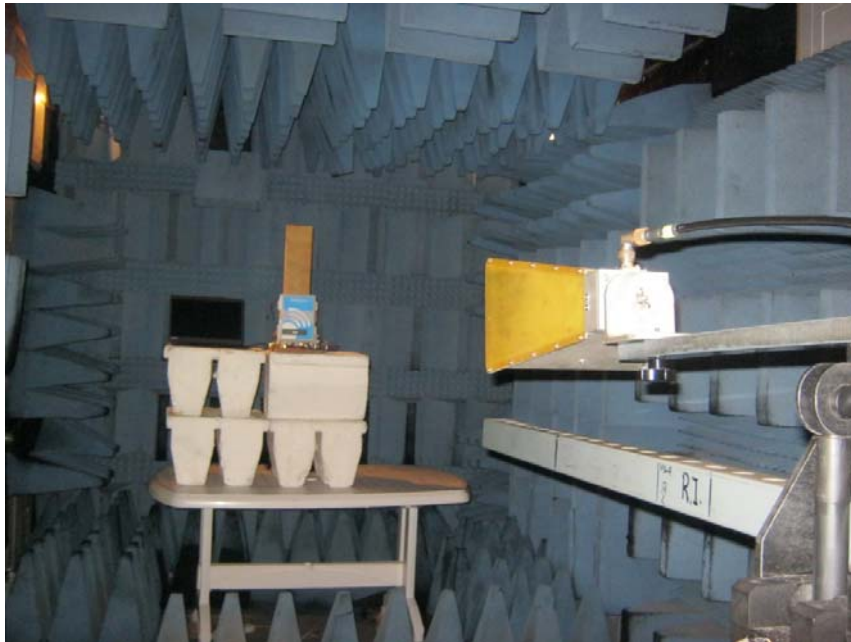
Figure 8. Radiated Emission Test, 1-18GHz
