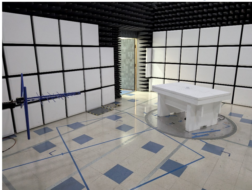
30-1000 MHz Radiated Emission Setup
