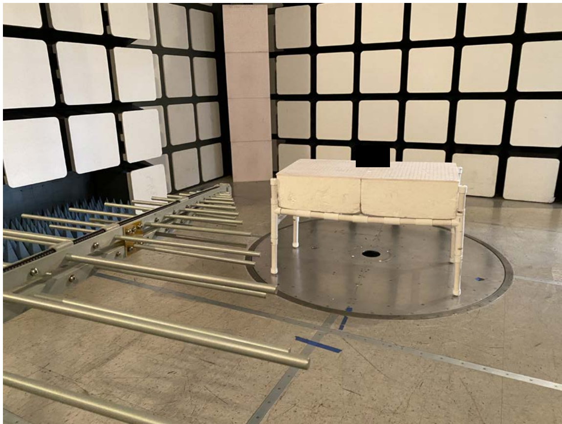
Box indicates position of EUT
