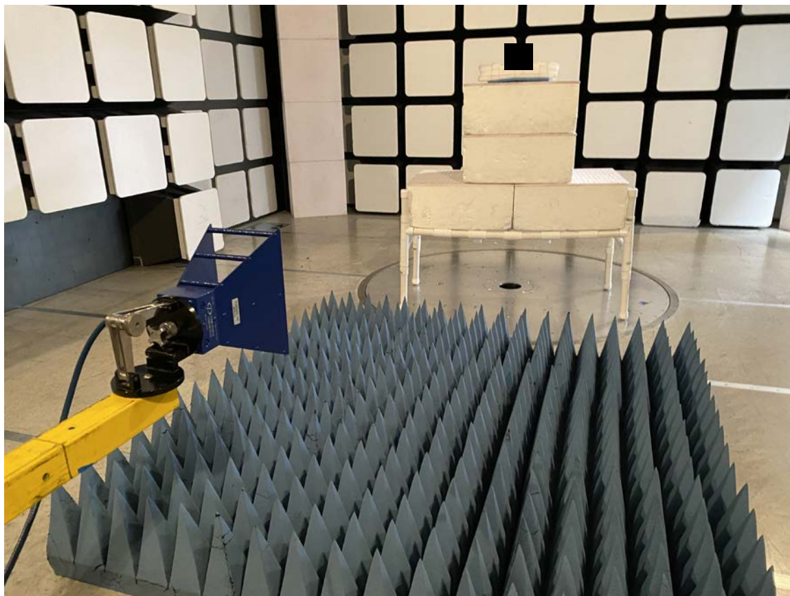
Box indicates position of EUT
