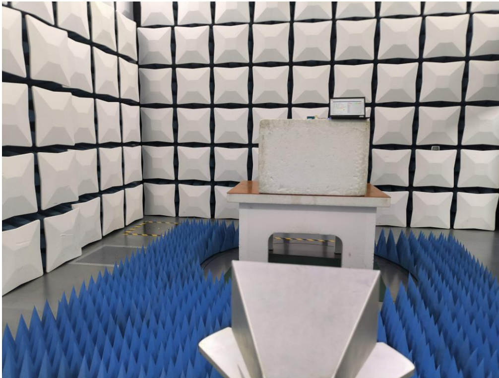
Test Set-up: Radiated spurious emission 1GHz to 18GHz
