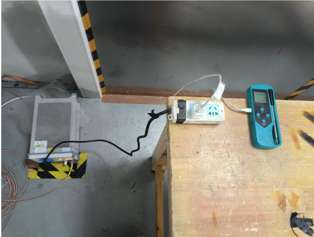
Test Set-up: Conducted emission 150KHz-30MHz
