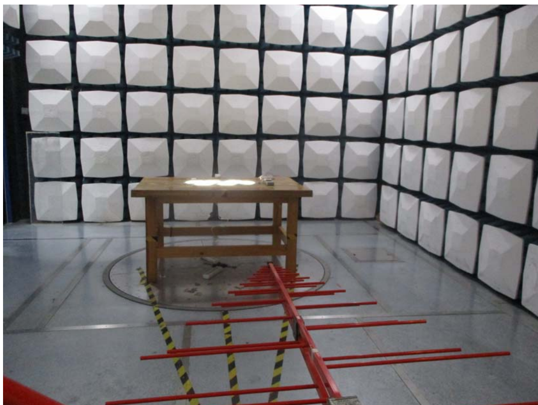
Radiated Emission Above 1GHz View
