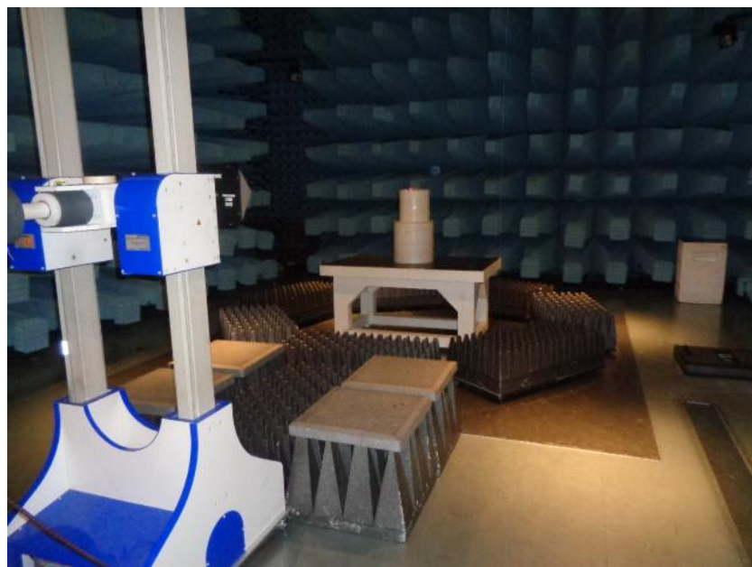
Figure 9.1-2: Radiated emissions set-up for frequencies above 1 GHz
