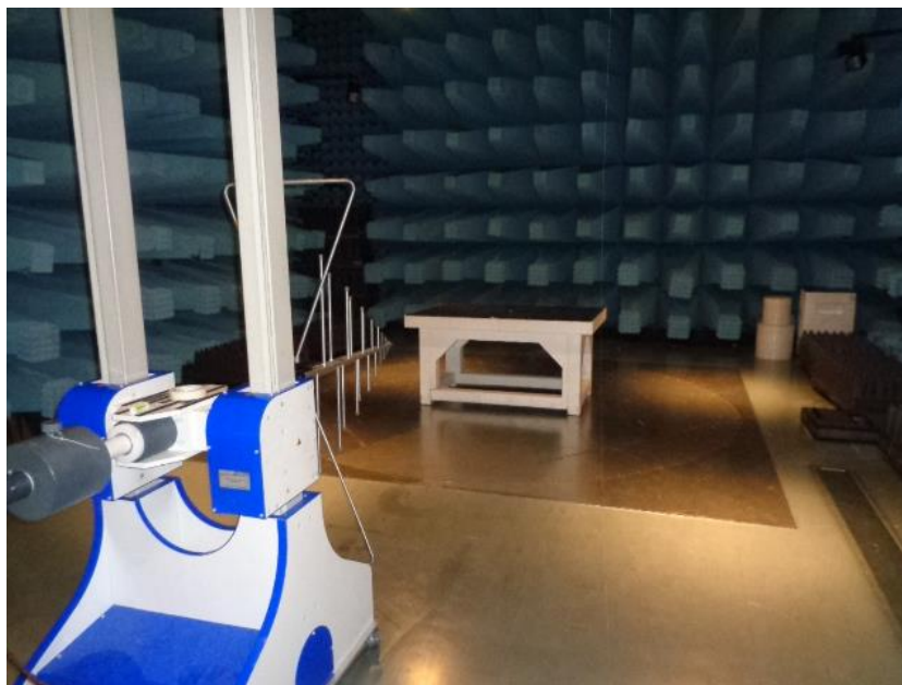
Figure 9.1-1: Radiated emissions set-up for frequencies below 1 GHz
