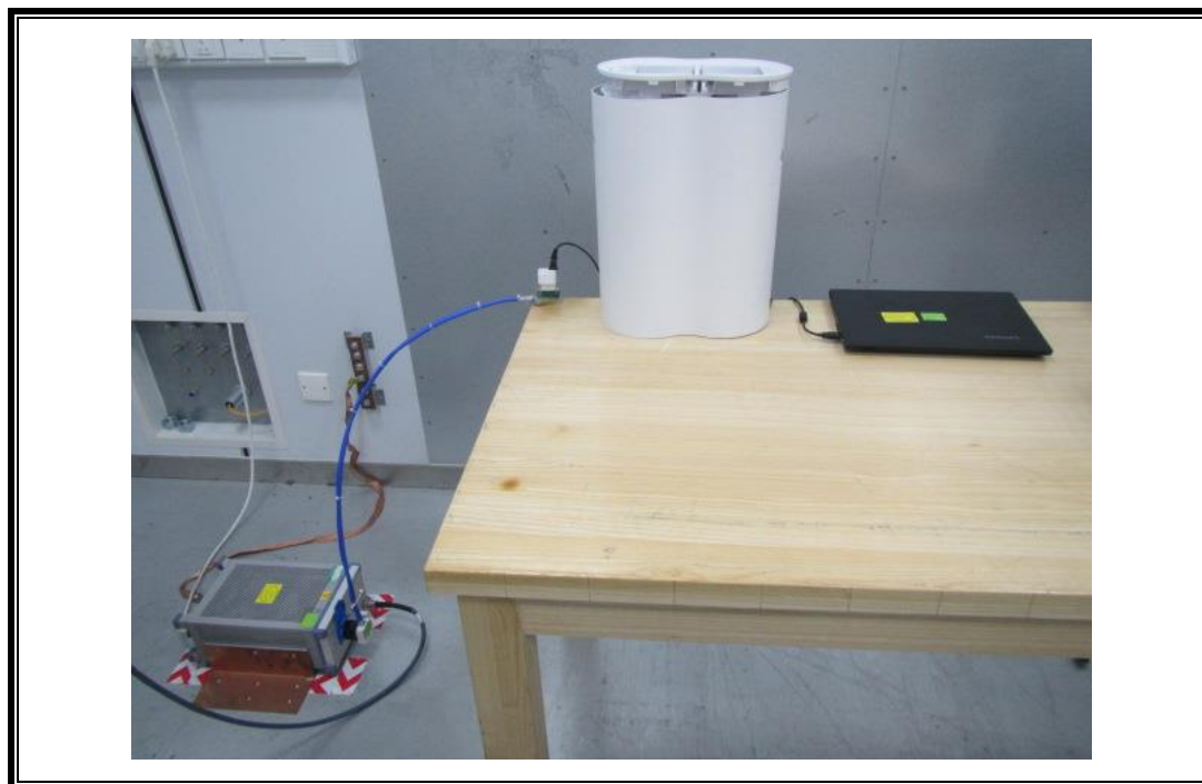
POWERLINE CONDUCTED EMISSIONS MEASUREMENT SETUP
