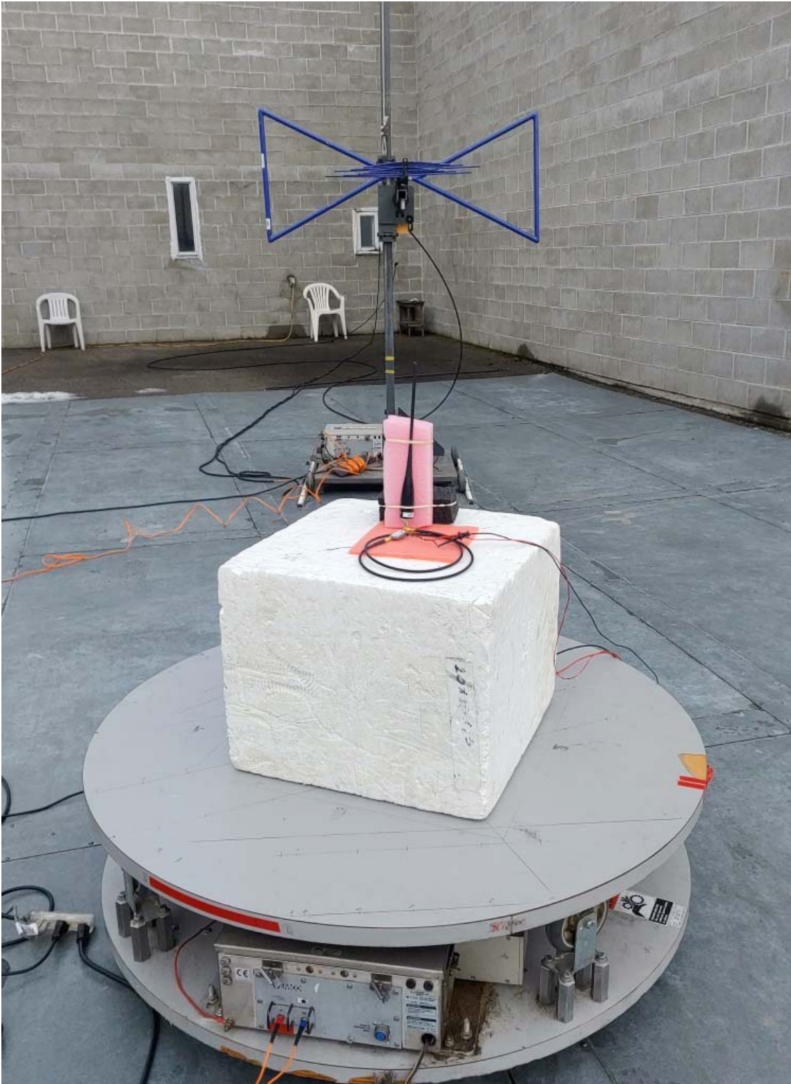
Figure E21.4 – Test Set Up - Radiated Measurements 30MHz – 1000MHz, Antenna #2
