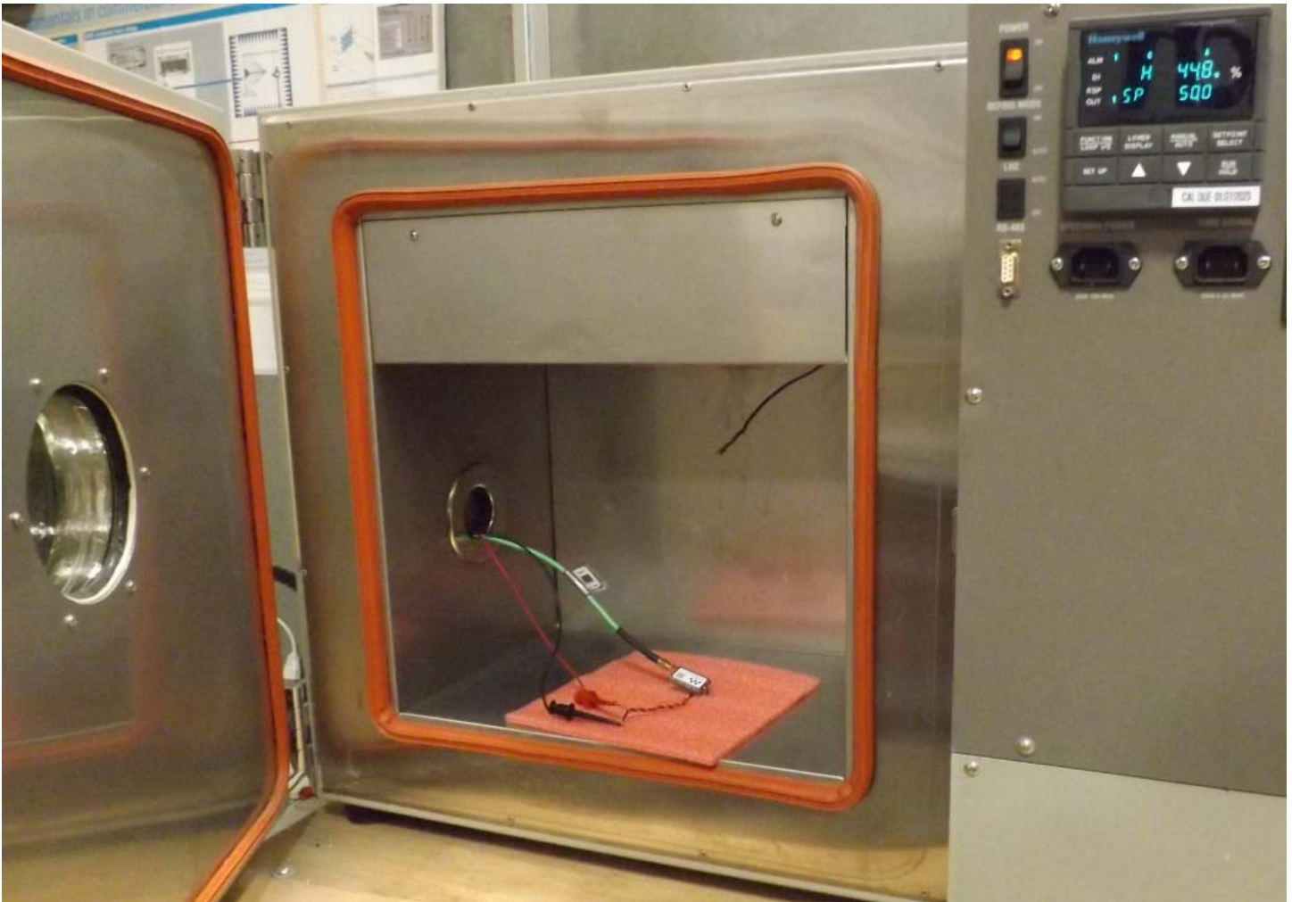
Figure E21.8 – Test Set Up - Frequency Stability
