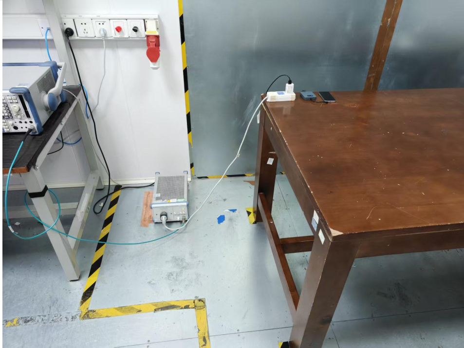
Conducted emissions at AC power line (150kHz-30MHz)
