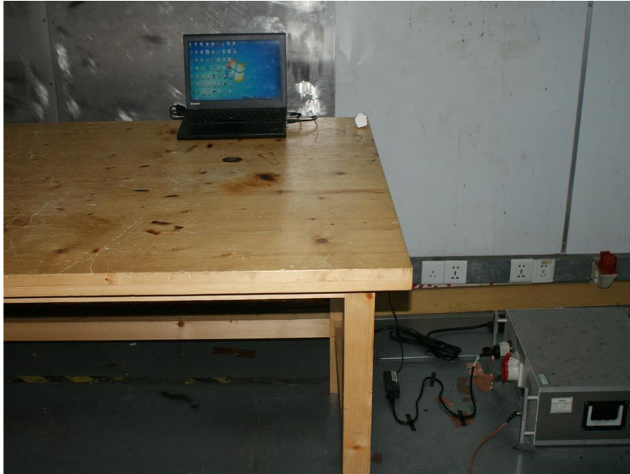
Photograph 1: Set-up for Conducted Emission on AC Mains
