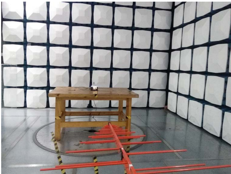
Radiated Emissions –Above 30MHz
