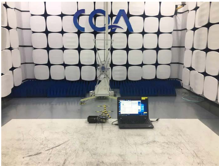
Radiated emission Test Setup-2 (30MHz~1GHz)
