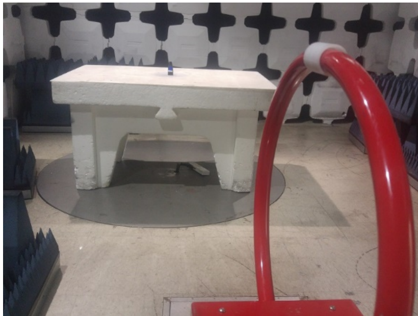
Photo 1. Radiated emissions test setup with Loop antenna.
