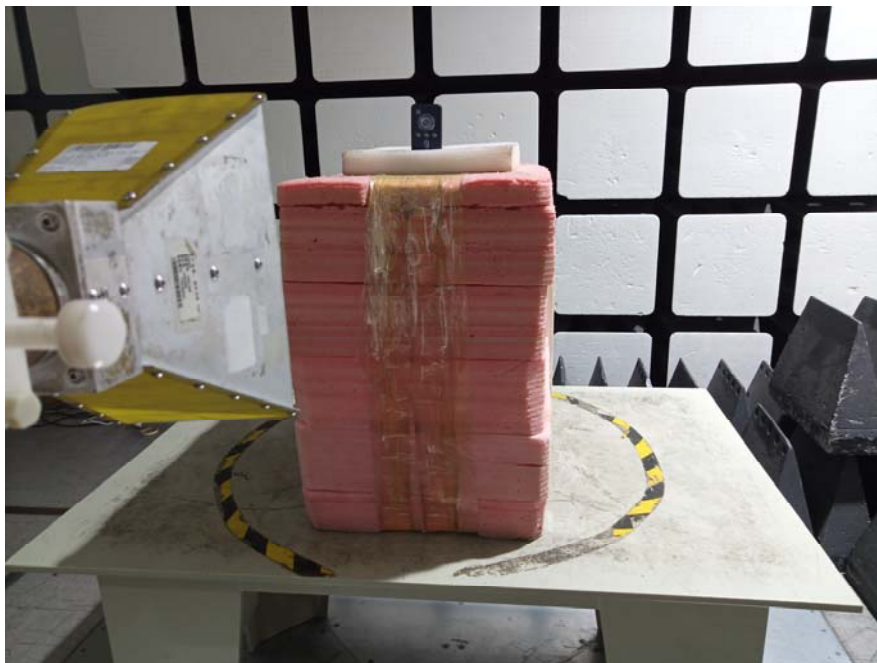
Radiated Emissions View (Above 1 GHz)
