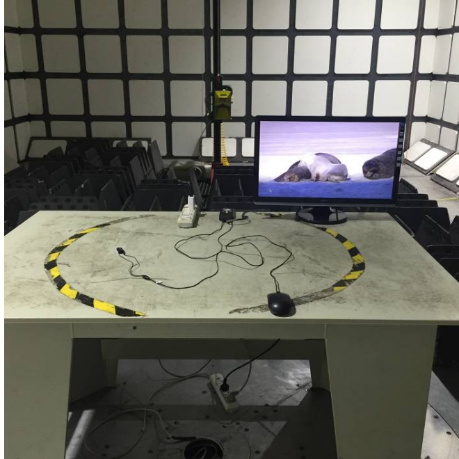
Radiated Emissions – Front View (Above 1 GHz)
