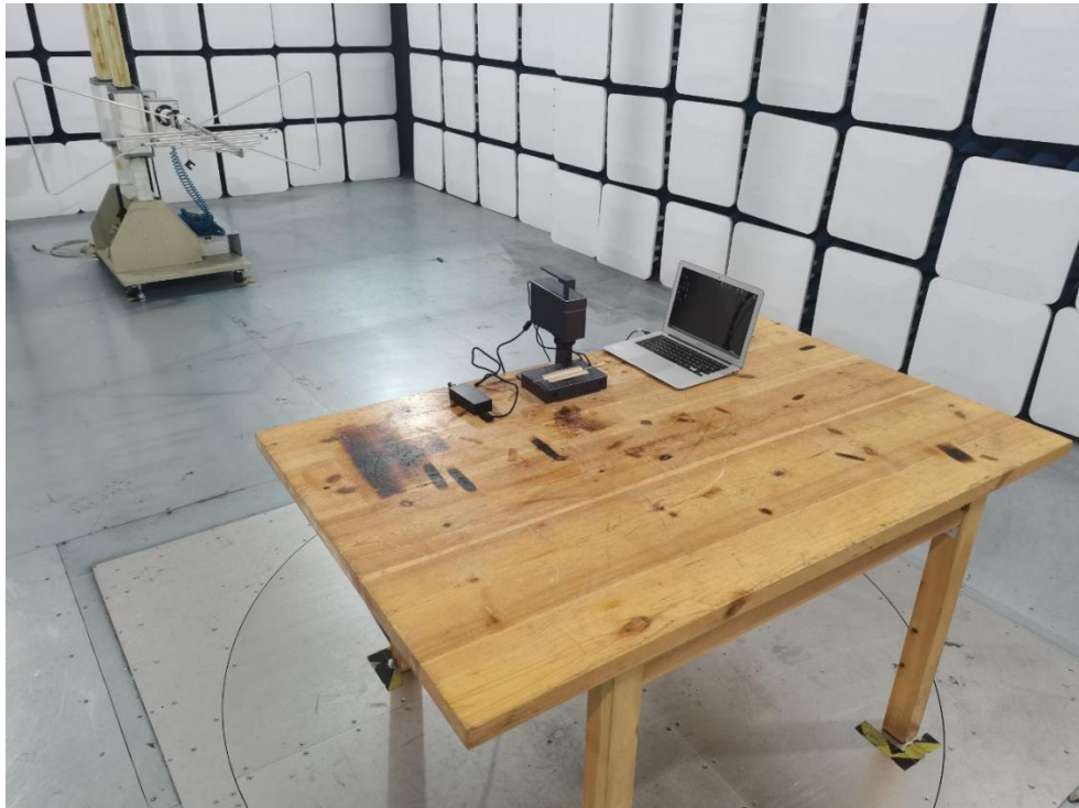
Photo of Radiation Emission Test
