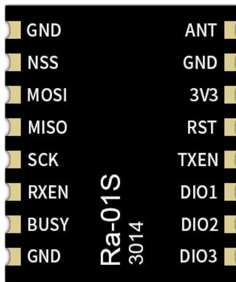
Ra-01SC Pin diagram
