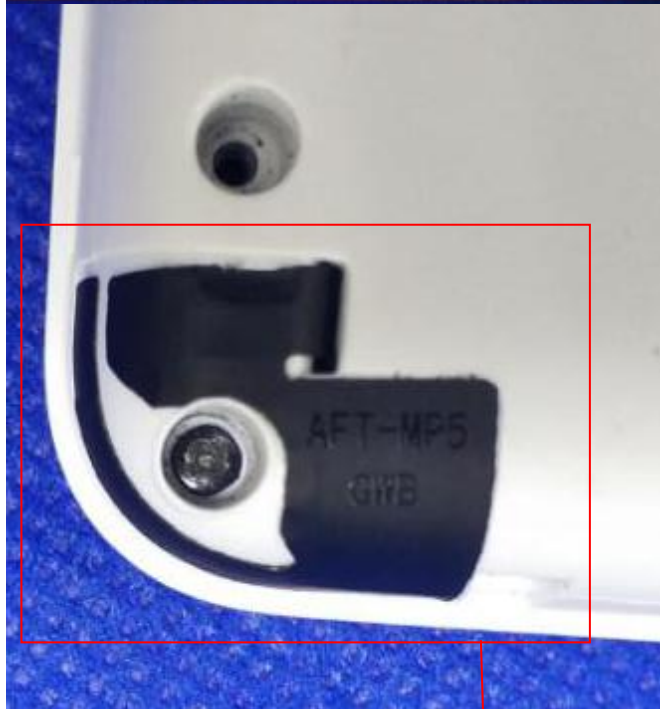
WiFi and BT in 1 antenna (External figure)
