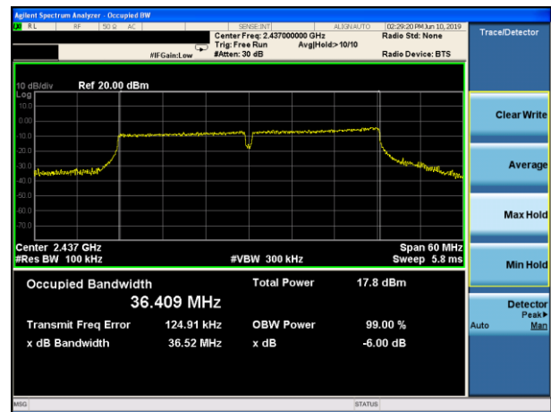
(802.11 N40) 6dB Bandwidth plot on channel 6
