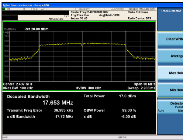
(802.11 N20) 6dB Bandwidth plot on channel 6
