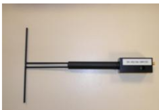
Figure 1 – MVG COMOSAR Validation Dipole
