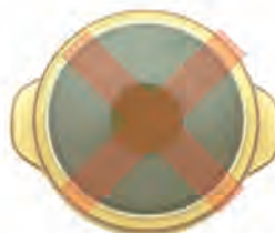
Even though magnetic field works, but cookware which is heated by thermal transfer film or spraying iron powder on bottom side
