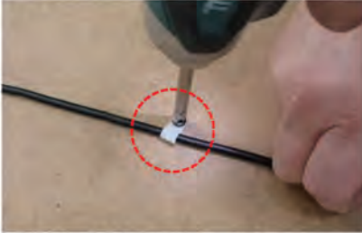
Fig.6 After fixing of control plate at table edge, organize lines with enclosed accessory and finish installation.
