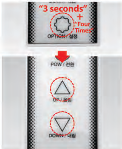
Fig.5 SET COMMUNICATION CHANNEL
