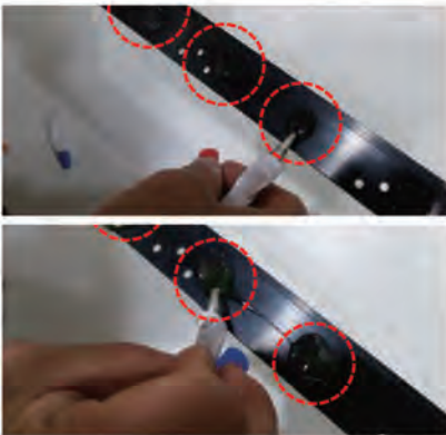
fig.4 Squeeze enclosed adhesive A and B as show in figure at same amount. (No matter the sequence of adhesives A / B)
