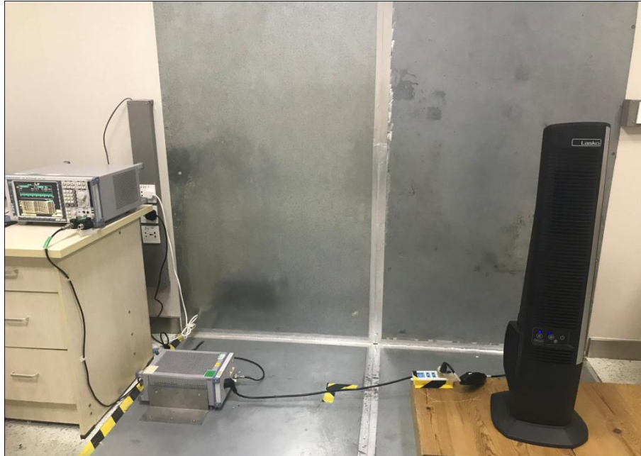
Radiated Spurious Emissions From 30MHz-1000MHz
