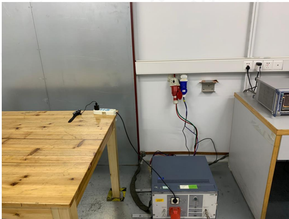
RADIATED EMISSION TEST SETUP BELOW 1GHZ
