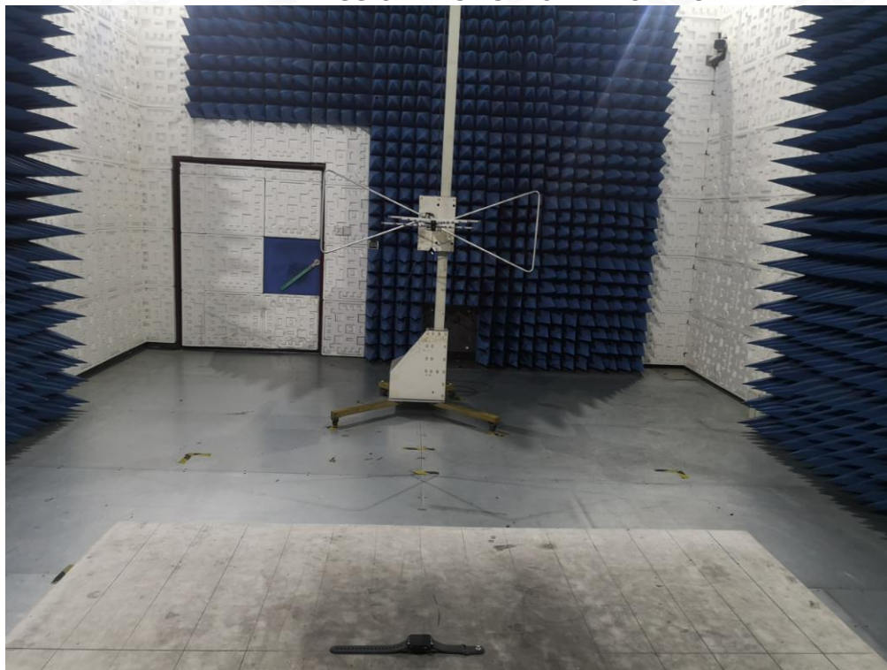
RADIATED EMISSION TEST SETUP BELOW 1GHZ
