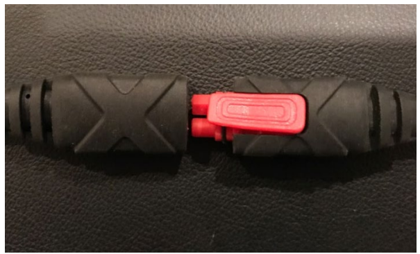
Figure 19 INCORRECT Insertion of Charger Plug
