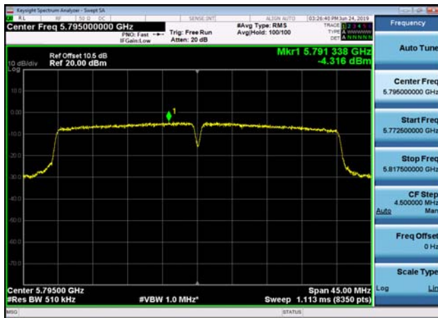
U-NII-3 Power spectral density-802.11 a(20MHz),5745MHz,Ant1
