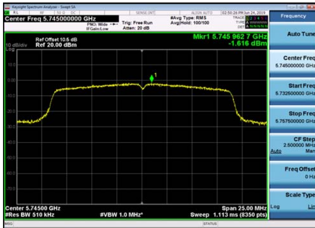
U-NII-3 Power spectral density-802.11 ac(20MHz),5785MHz,Ant1
