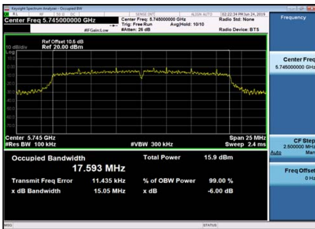
U-NII-3 6dB Bandwidth-802.11n(20MHz) ,5745MHz,Ant1
