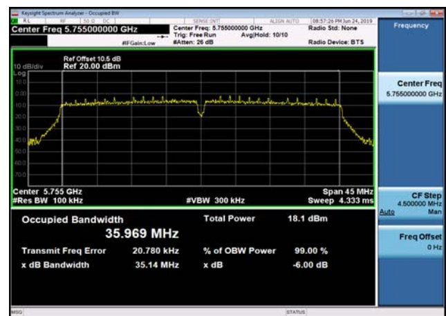
U-NII-3 6dB Bandwidth-802.11n(40MHz) ,5755MHz,Ant2
