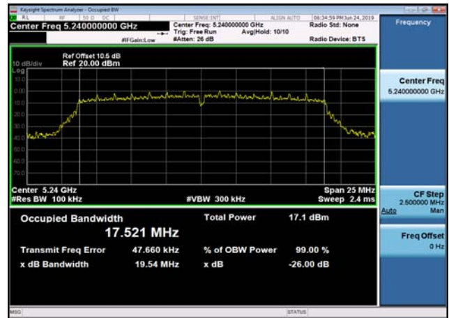
U-NII-1 26dB Bandwidth-802.11ac(40MHz ,5190MHz,Ant2
