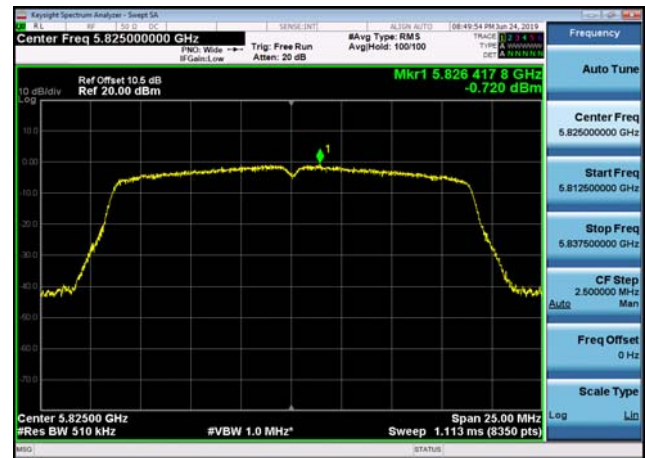
U-NII-3 Power spectral density-802.11 ac(40MHz),5755MHz,Ant2
