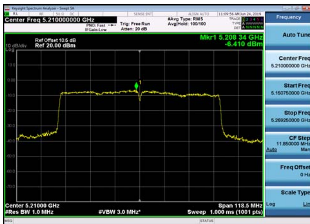
U-NII-3 Power spectral density-802.11 n(20MHz),5745MHz,Ant1
