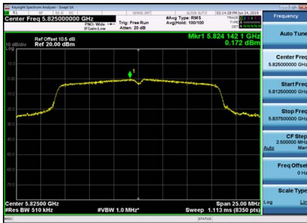
U-NII-3 Power spectral density-802.11 ac(20MHz),5745MHz,Ant1
