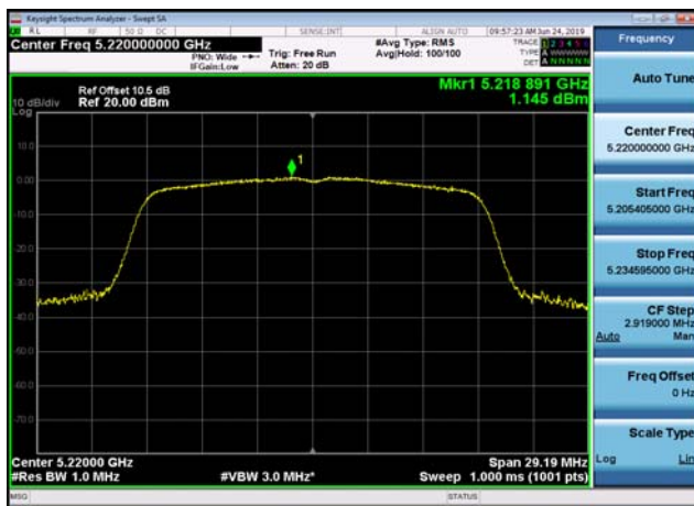
U-NII-1 Power spectral density-802.11 ac(20MHz),5240MHz,Ant1
