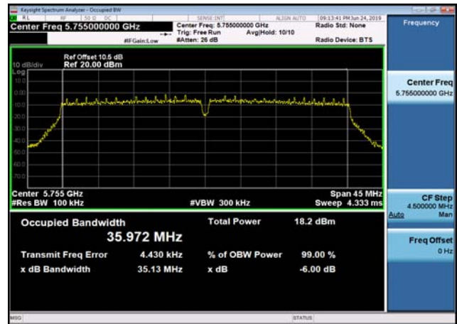
U-NII-3 6dB Bandwidth-802.11ac(40MHz) ,5795MHz,Ant2
