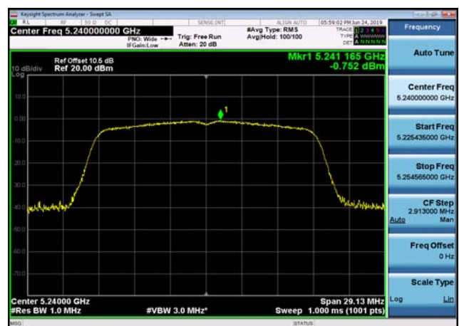
U-NII-1 Power spectral density-802.11 n(20MHz),5240MHz,Ant2
