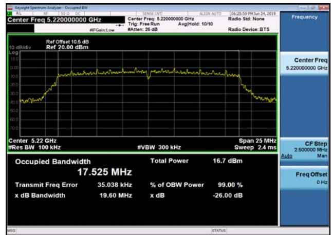
U-NII-1 26dB Bandwidth-802.11ac(20MHz ,5240MHz,Ant2
