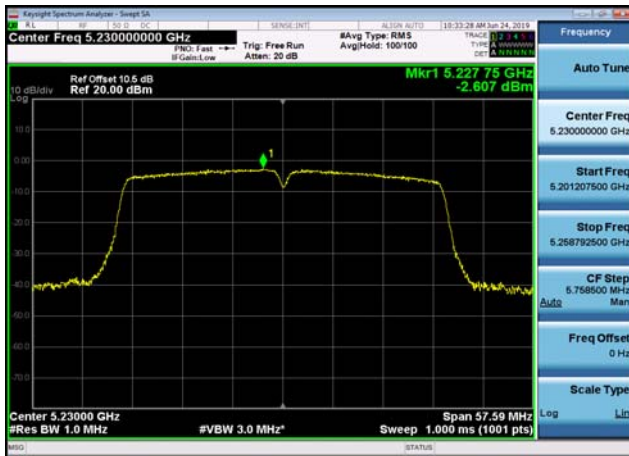
U-NII-1 Power spectral density-802.11 a(20MHz),5180MHz,Ant1
