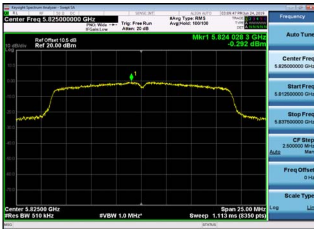
U-NII-3 Power spectral density-802.11 ac(40MHz),5755MHz,Ant1
