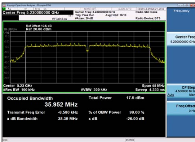
U-NII-1 26dB Bandwidth-802.11a(20MHz) ,5180MHz,Ant1
