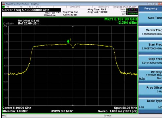
U-NII-1 Power spectral density-802.11 n(40MHz),5230MHz,Ant1
