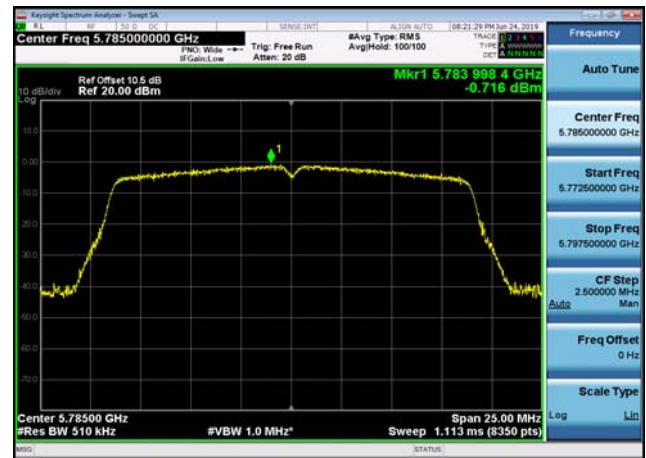
U-NII-3 Power spectral density-802.11 n(20MHz),5825MHz,Ant2
