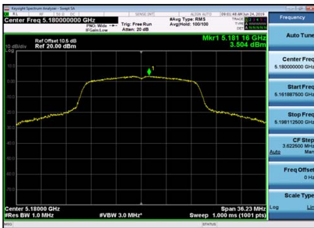
U-NII-1 Power spectral density-802.11 a(20MHz),5180MHz,Ant1
