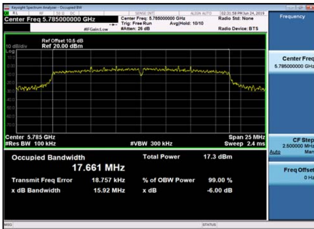
U-NII-3 6dB Bandwidth-802.11n(20MHz) ,5825MHz,Ant1
