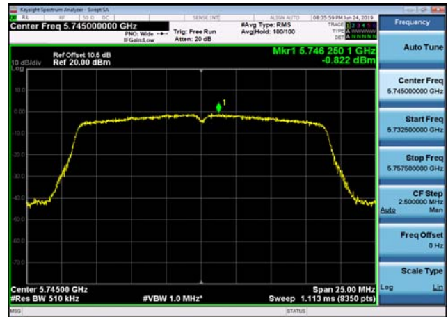
U-NII-3 Power spectral density-802.11 ac(20MHz),5785MHz,Ant2
