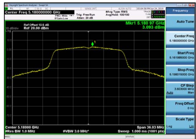
U-NII-1 Power spectral density-802.11 a(20MHz),5180MHz,Ant2
