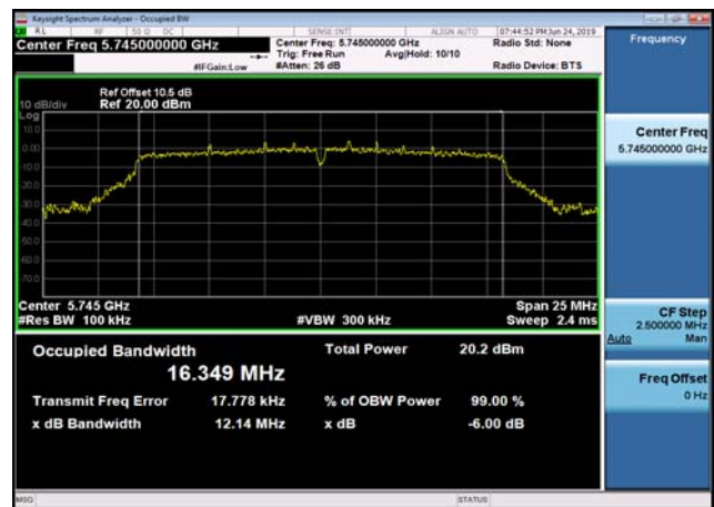
U-NII-3 6dB Bandwidth-802.11a(20MHz) ,5785MHz,Ant2
