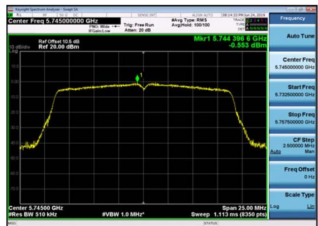
U-NII-3 Power spectral density-802.11 n(20MHz),5745MHz,Ant2
