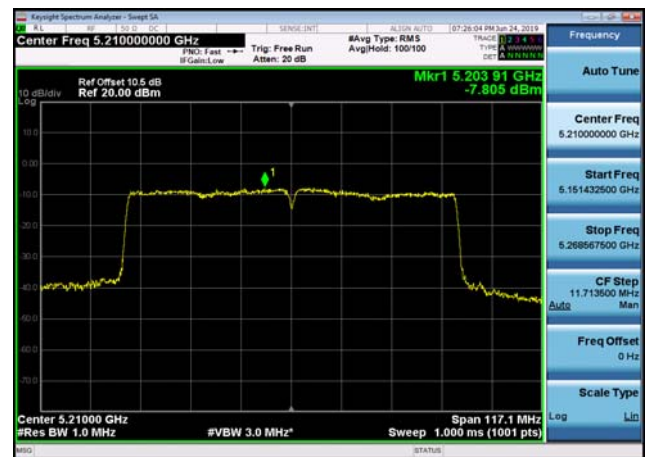
U-NII-3 Power spectral density-802.11 n(20MHz),5745MHz,Ant2
