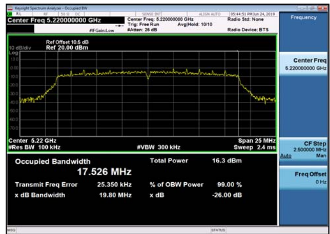
U-NII-1 26dB Bandwidth-802.11n(20MHz) ,5240MHz,Ant2
