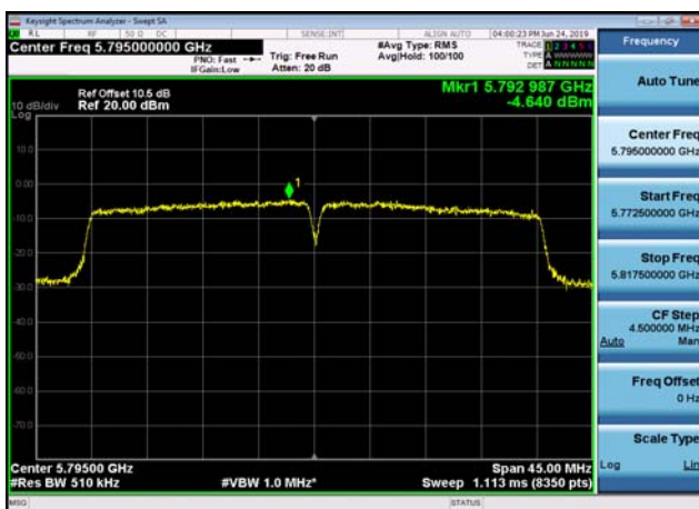
U-NII-3 Power spectral density-802.11 ac(40MHz),5795MHz,Ant1
