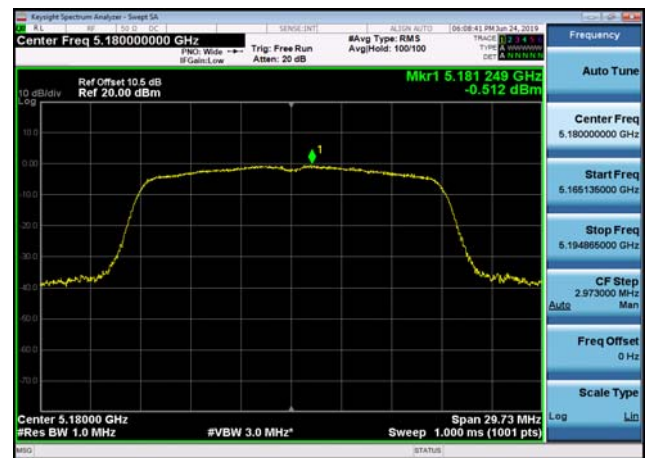
U-NII-1 Power spectral density-802.11 ac(20MHz),5180MHz,Ant2
