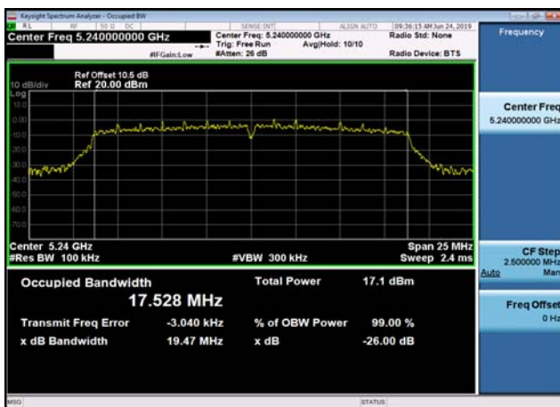
U-NII-1 26dB Bandwidth-802.11n(20MHz) ,5240MHz,Ant1
