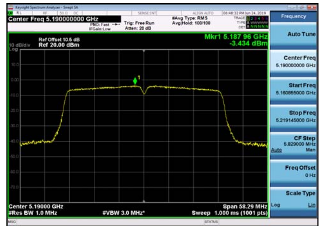
U-NII-1 Power spectral density-802.11 n(40MHz),5230MHz,Ant2
