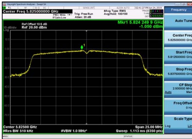
U-NII-3 Power spectral density-802.11 n(40MHz),5755MHz,Ant1
