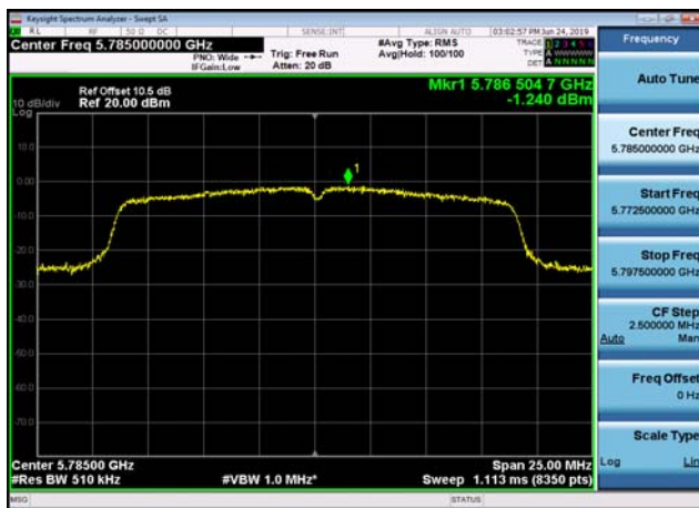
U-NII-3 Power spectral density-802.11 ac(20MHz),5785MHz,Ant1
