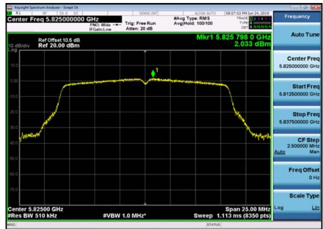
U-NII-3 Power spectral density-802.11 ac(20MHz),5745MHz,Ant2
