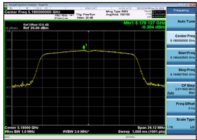
U-NII-1 Power spectral density-802.11 n(20MHz),5220MHz,Ant2
