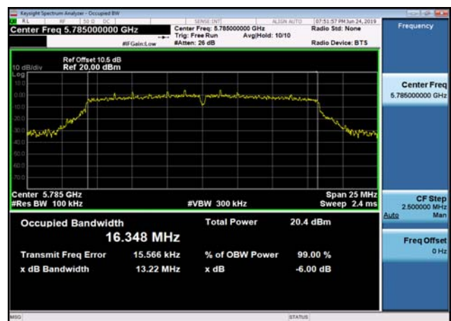
U-NII-3 6dB Bandwidth-802.11a(20MHz) ,5785MHz,Ant2
