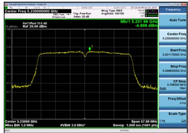
U-NII-1 Power spectral density-802.11 ac(80MHz),5210MHz,Ant2
