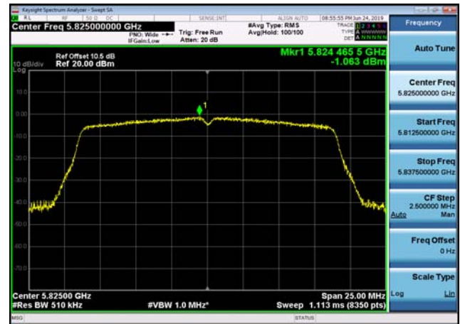
U-NII-3 Power spectral density-802.11 n(40MHz),5755MHz,Ant2
