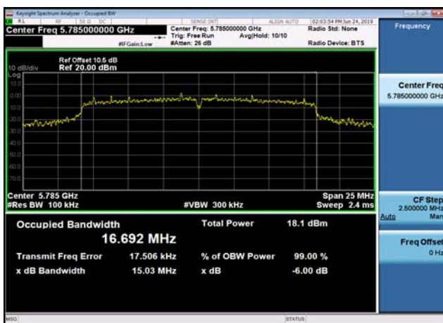
U-NII-3 6dB Bandwidth-802.11a(20MHz) ,5785MHz,Ant1
