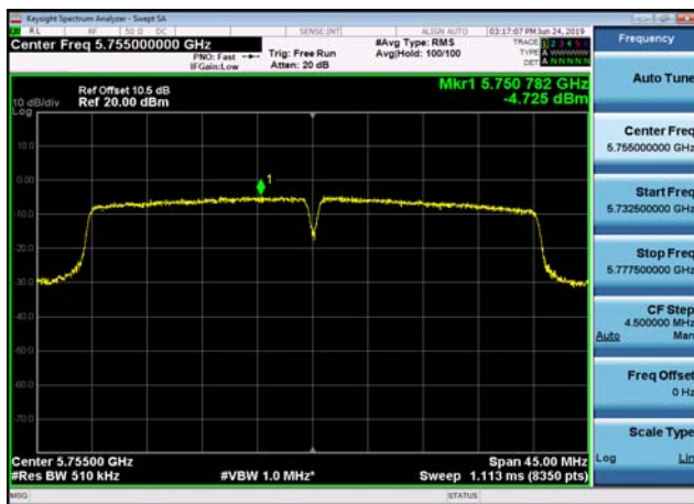
U-NII-3 Power spectral density-802.11 n(40MHz),5755MHz,Ant1
