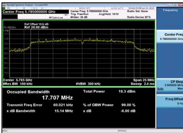
U-NII-3 6dB Bandwidth-802.11ac(20MHz) ,5785MHz,Ant1
