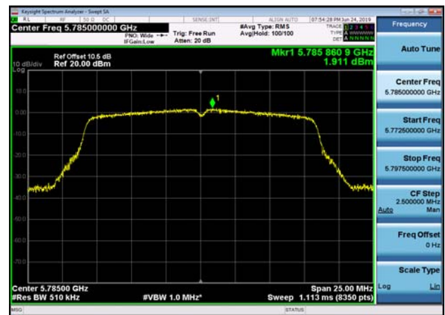
U-NII-3 Power spectral density-802.11 a(20MHz),5785MHz,Ant2
