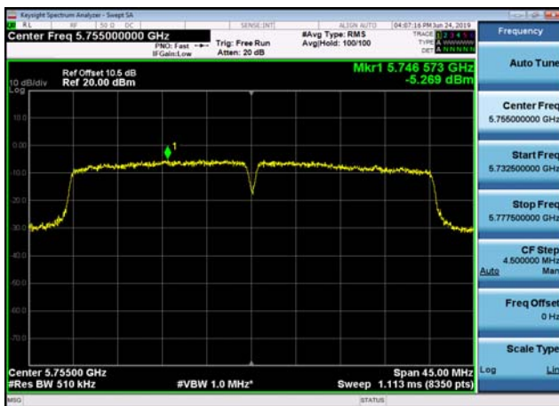
U-NII-3 Power spectral density-802.11 ac(40MHz),5795MHz,Ant1
