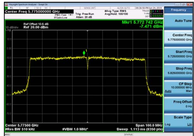
U-NII-3 Power spectral density-802.11 ac(80MHz),5775MHz,Ant2
