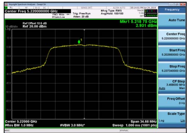
U-NII-1 Power spectral density-802.11 a(20MHz),5240MHz,Ant2
