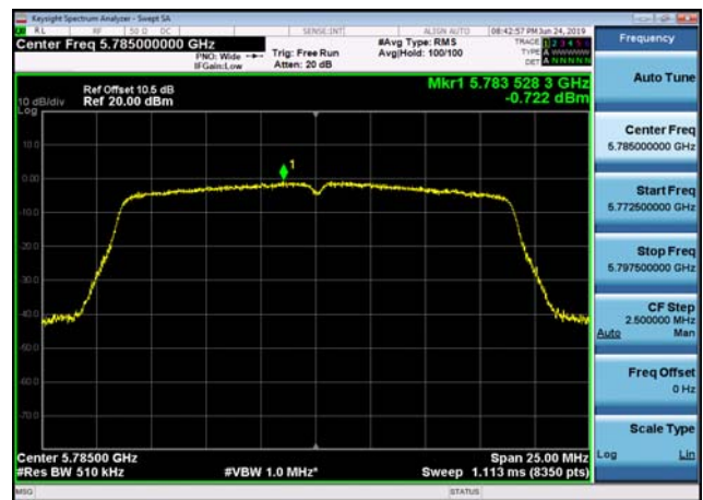
U-NII-3 Power spectral density-802.11 ac(20MHz),5785MHz,Ant2
