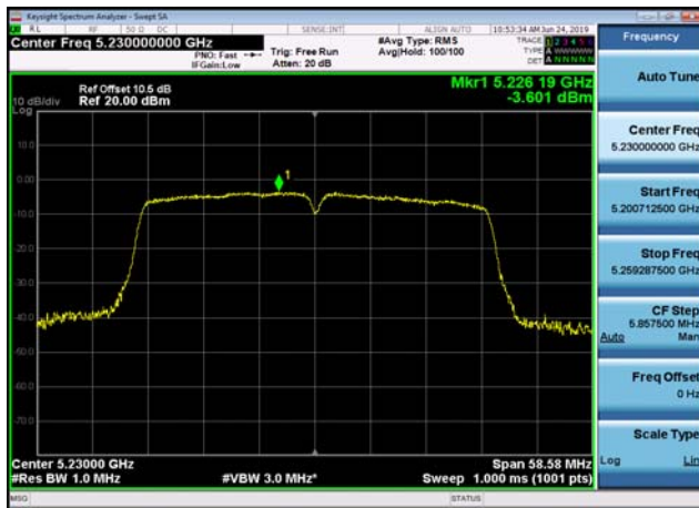
U-NII-1 Power spectral density-802.11 ac(80MHz),5210MHz,Ant1
