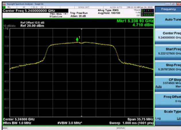
U-NII-1 Power spectral density-802.11 ac(20MHz),5180MHz,Ant1
