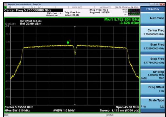
U-NII-3 Power spectral density-802.11 n(40MHz),5755MHz,Ant2
