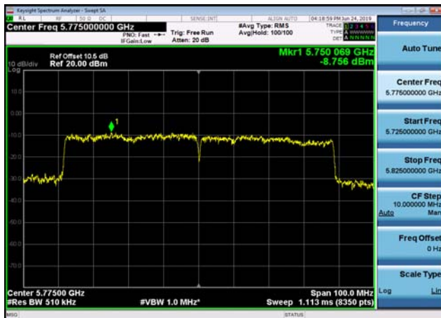
U-NII-3 Power spectral density-802.11 ac(80MHz),5775MHz,Ant1
