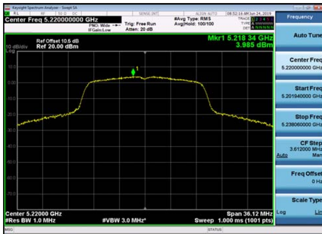
U-NII-1 Power spectral density-802.11 a(20MHz),5240MHz,Ant1
