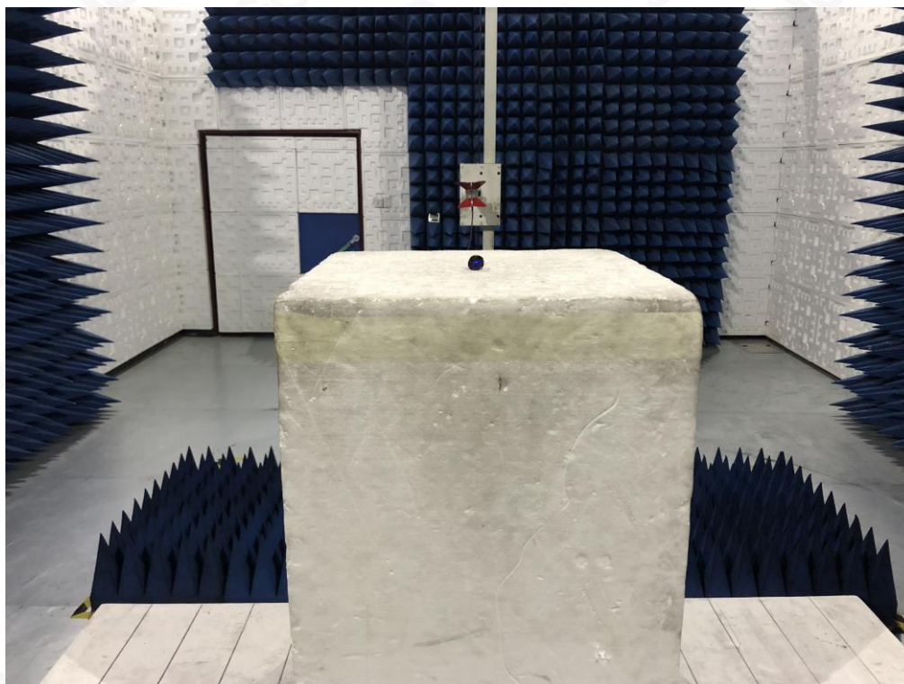
RADIATED EMISSION TEST SETUP ABOVE 1GHZ
