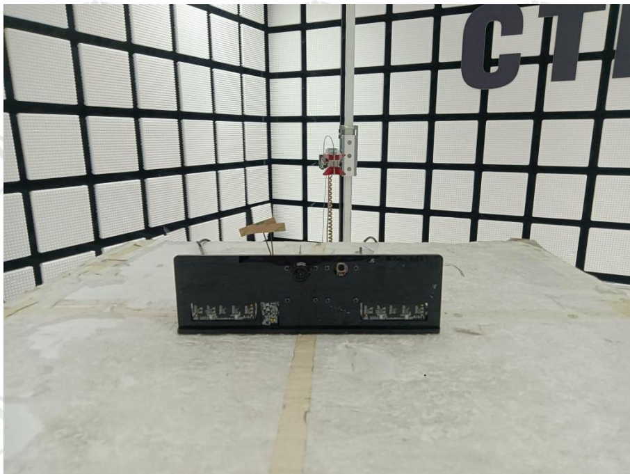
Radiated spurious emission Test Setup-2(Above 1GHz)
