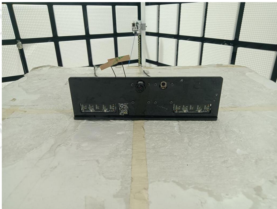
Radiated spurious emission Test Setup-3(Above 18GHz)
