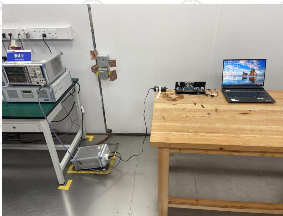
Conducted emission Test Setup
