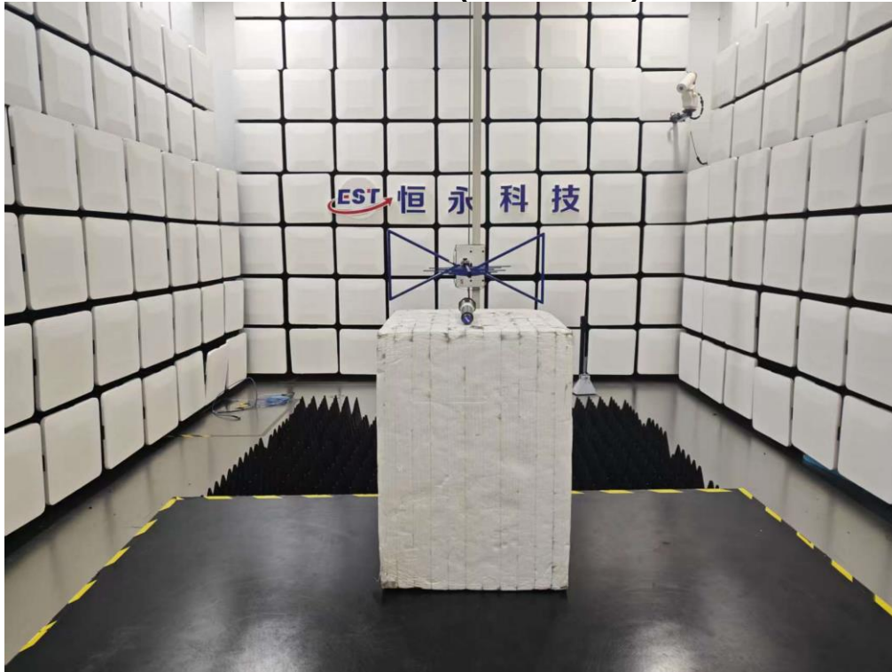
Radiated Test (Below 1GHz)
