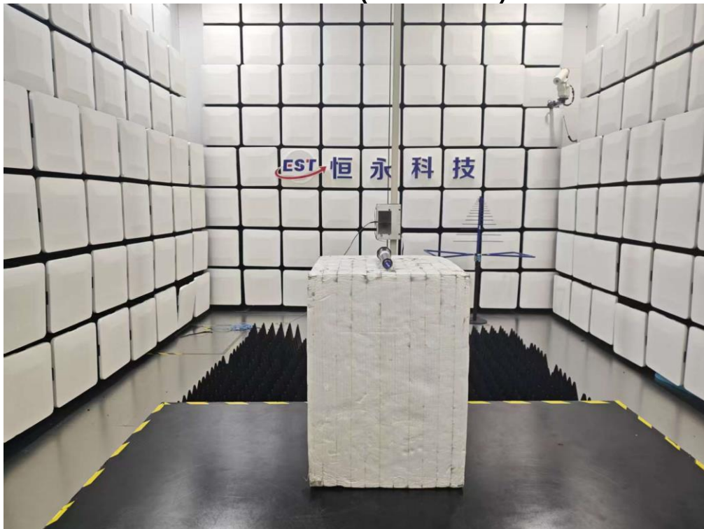
Radiated Test (Above 1GHz)
