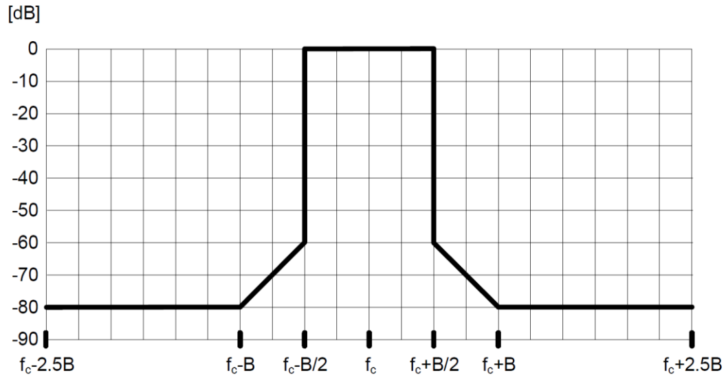
Figure 1: Transmit spectral power mask for equipment employing analogue modulation, RBW = 1 kHz
