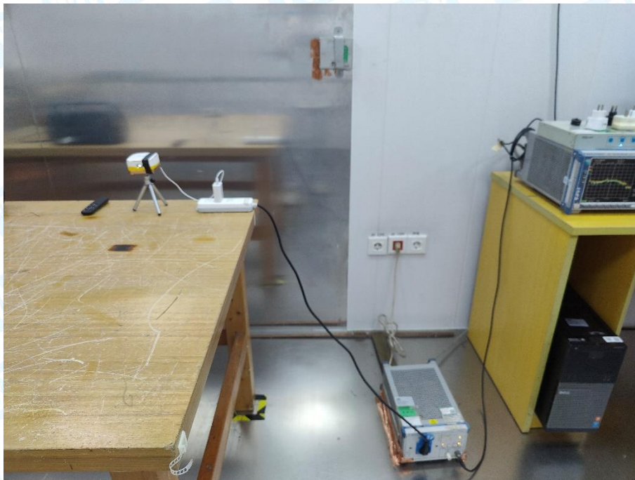
Photo of Setup for Conducted Emission
