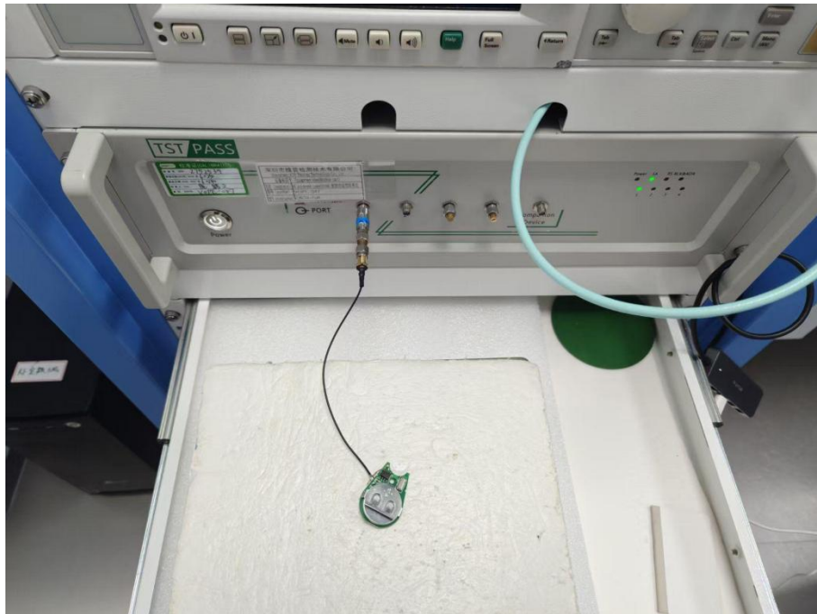
Conducted RF test
