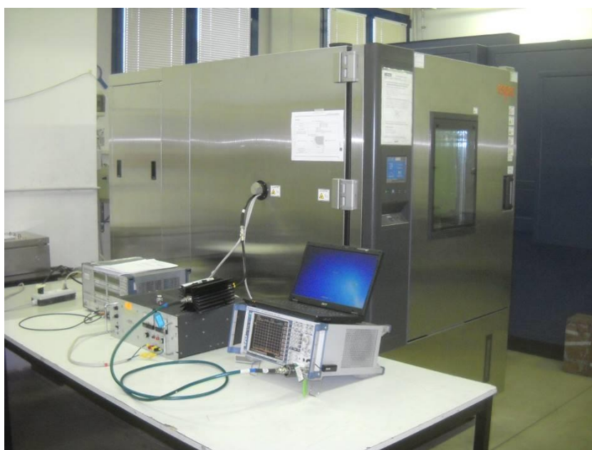
Set-up photo for frequency error tests
