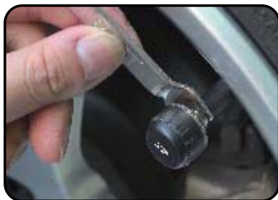
Reverse fixed sensors and screw
