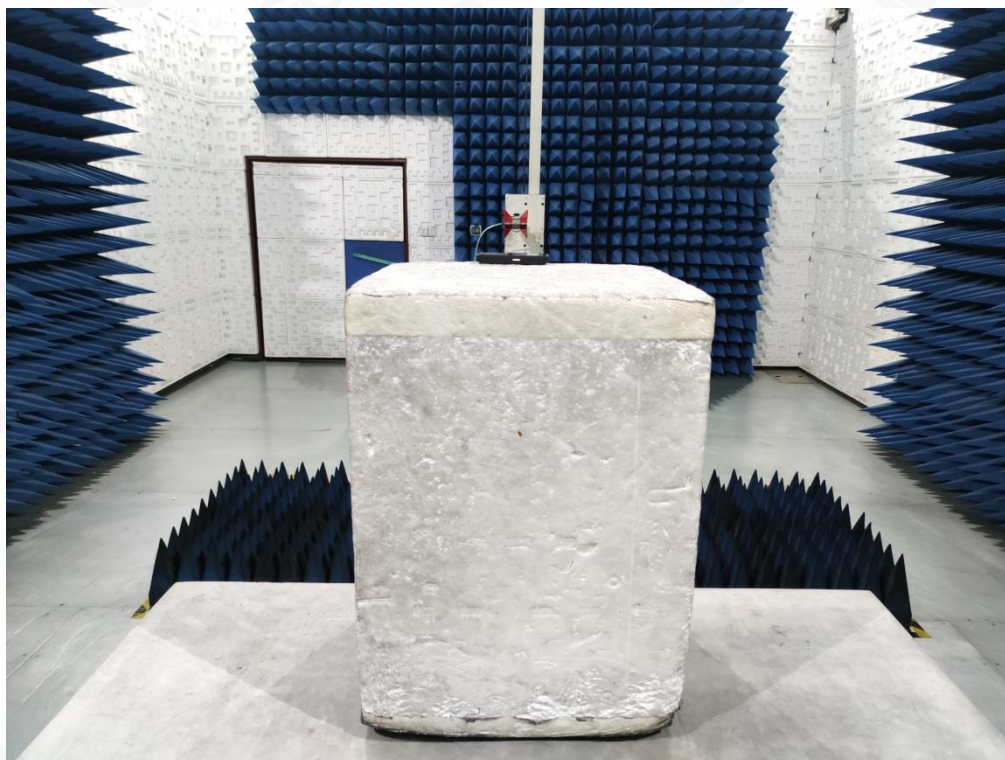
FCC RADIATED EMISSION TEST SETUP ABOVE 1GHZ
