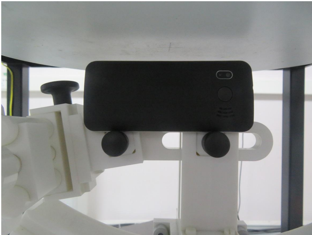
10mm body-worn Right Side Setup Photo (hotspot)
