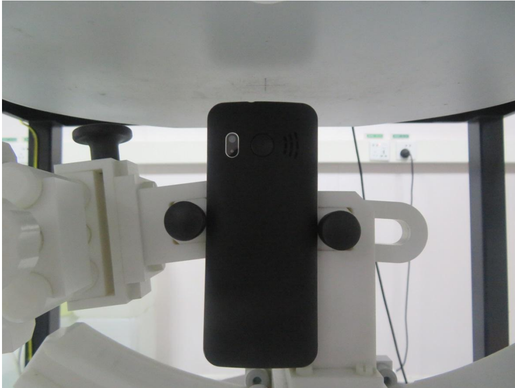
10mm body-worn Bottom Side Setup Photo (hotspot)
