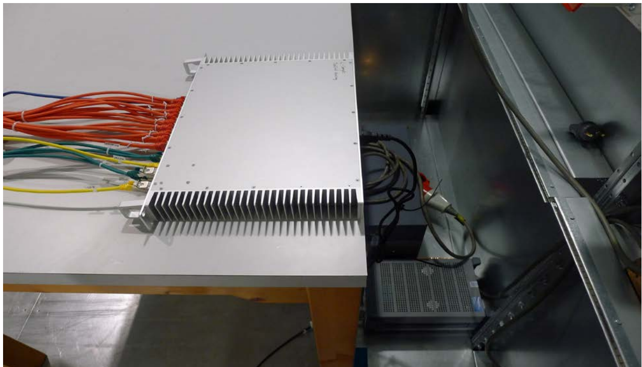
Photo 4: Setup in the Test room 1 Conducted emissions measurement at AC power lines (150 kHz – 30 MHz)
