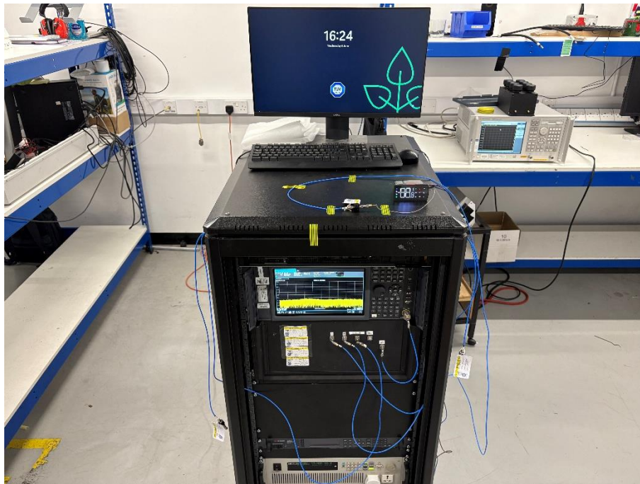
Figure 36 - Test Setup for Maximum Conducted Output Power, Power Spectral Density and Emission Bandwidth.
