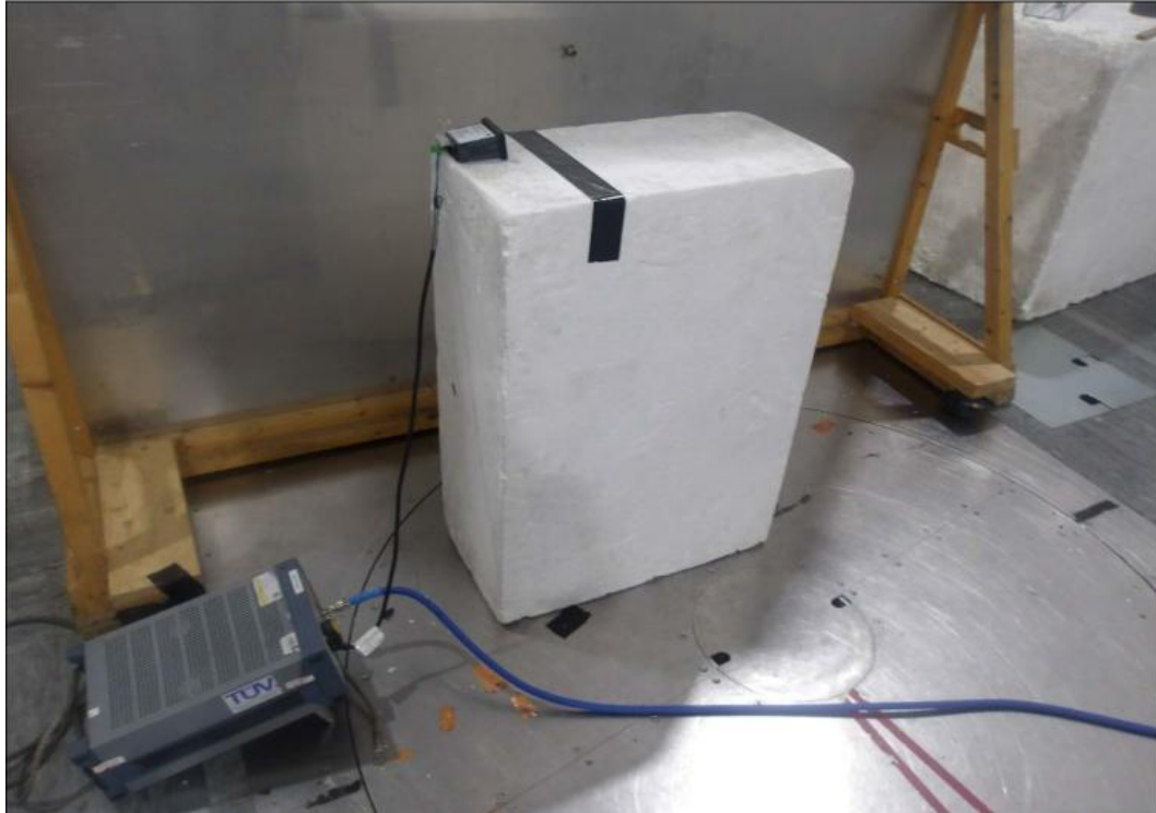
Figure 1 - AC Line Power Conducted Emissions
