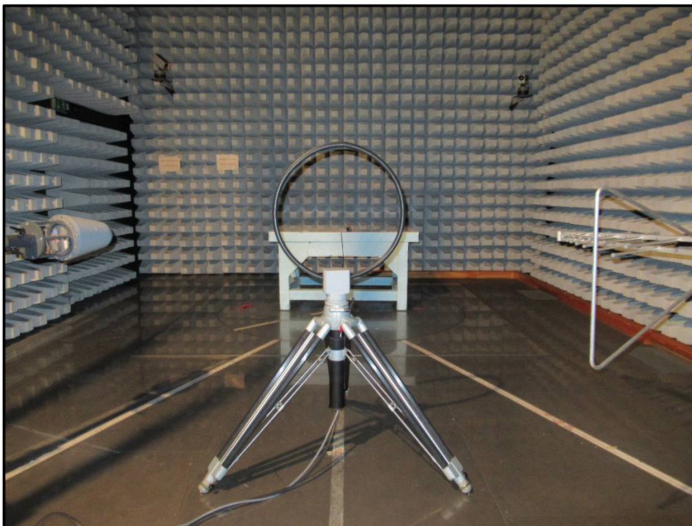
Photo 1: Radiated Test Setup-9 kHz to 30 MHz
