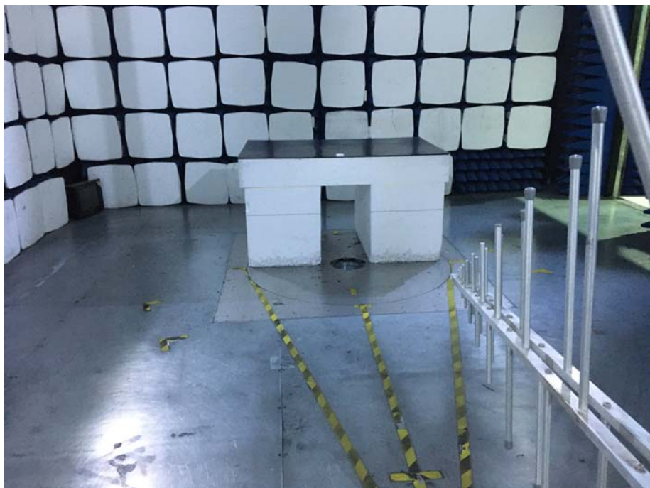
Radiation Emission Test Setup (30MHz to 1GHz)
