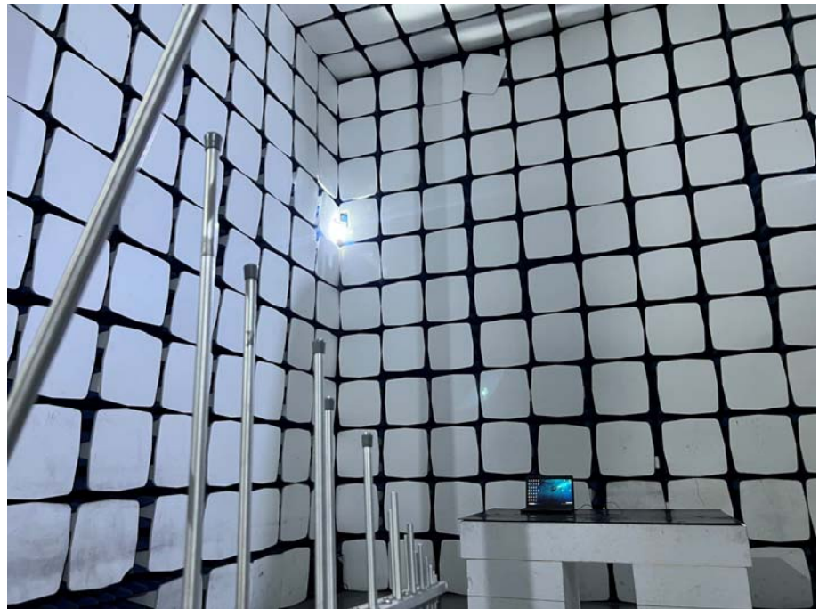
Radiation Emission Test Setup (30MHz to 1GHz)
