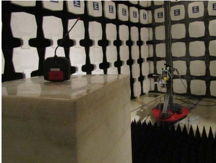
Measurement of Radiated Emission Test Set Up
