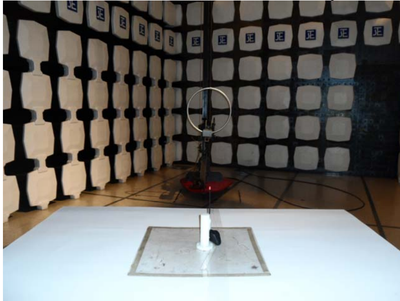
Measurement of Radiated Emission Test Set Up
