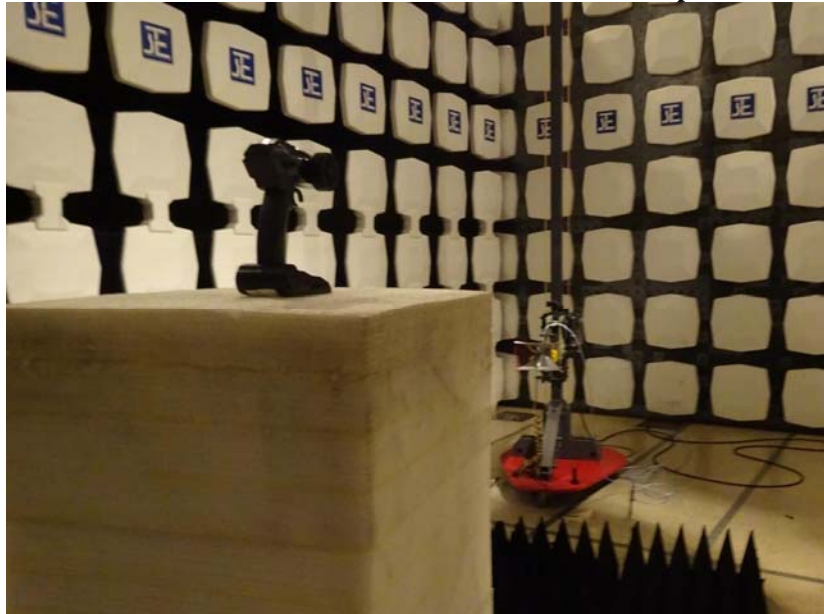
Measurement of Radiated Emission Test Set Up
